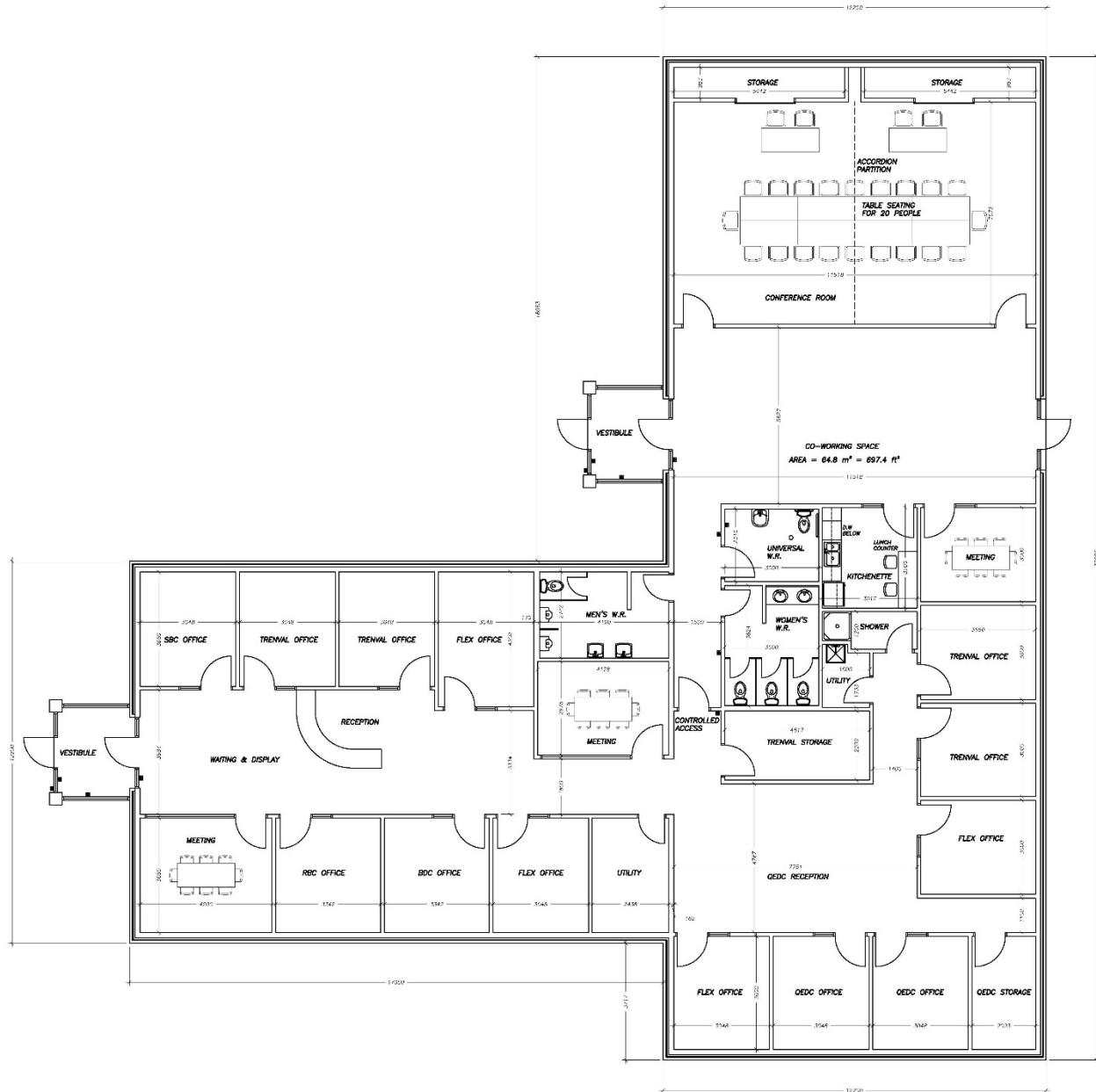
Figure 3 – Concept Building Plan prepared by R. Morden Engineering & Contracting Ltd., dated March 25, 2020 illustrates how the proposed 600m 2 office building on the subject lands would function.
