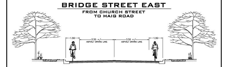
The proposed widths for bike and motor vehicle lanes on Bridge Street East are consistent with design guidelines.
